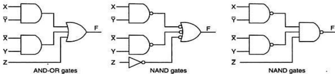
Two –level implementation using AND-OR and NAND logic
