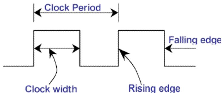
From the diagram you can see that the **clock period** is the time between successive transitions in the same direction, that is, between two rising or two falling edges. State transitions in synchronous sequential circuits are made to take place at times when the clock is making a transition from 0 to 1 (rising edge) or from 1 to 0 (falling edge). Between successive clock pulses there is no change in the information stored in memory.
