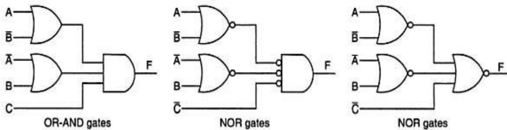
Two –level implementation using OR-AND and NOR logic
