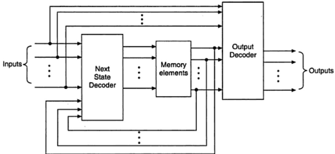
**Moore model:** when the output of the sequential circuit depends up only on the present state of the flip-flop, the sequential circuit is referred as to as the Moore circuit or the Moore machine.
