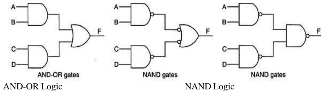
Two –level implementation using AND-OR and NAND logic
