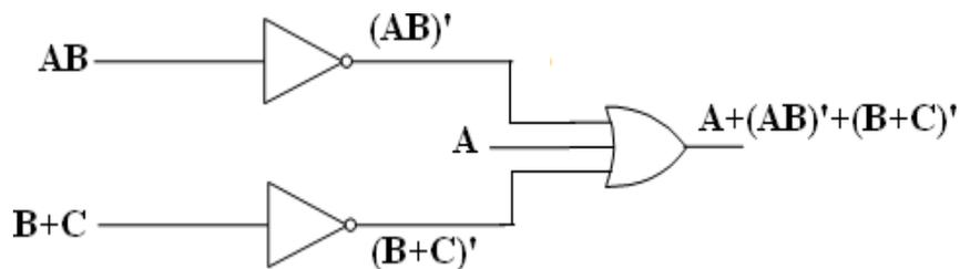
Now  $AB$  must be output of a two-input AND gate whose inputs are  $A$  and  $B$ . And  $B+C$  must be the output of a two-input OR gate whose inputs are  $B$  and  $C$ . so, an AND gate and an OR gate are as
