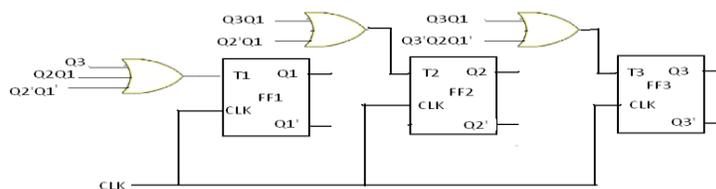
**Design of a synchronous BCD Up-Down counter using FFs:**
