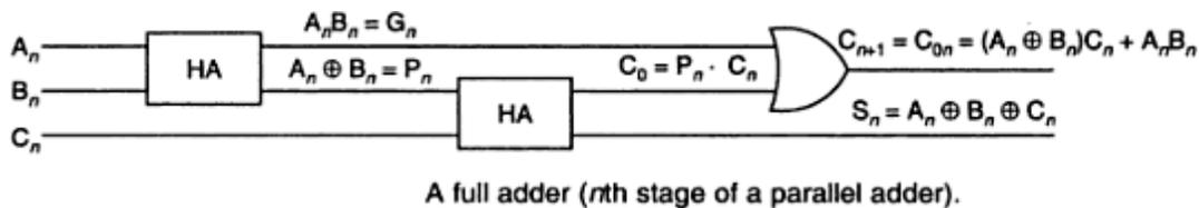
There is another possibility of producing a carry out. X-OR gate inside the half-adder at the input produces an intermediary sum bit- call it  $P_n$  –which is expressed as  $P_n = A_n \oplus B_n$ . Next  $P_n$  and  $C_n$  are added using the X-OR gate inside the second half adder to produce the final
