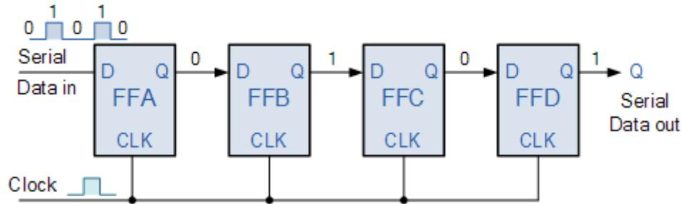
When serial data is transferred into a register, each new bit is clocked into the first FF at the positive going edge of each clock pulse. The bit that was previously stored by the first FF is transferred to the second FF. the bit that was stored by the Second FF is transferred to the third FF.
