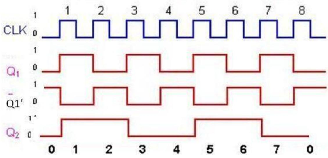
A 2-bit down-counter counts in the order 0,3,2,1,0,1.....,i.e, 00,11,10,01,00,11 .....etc. the above fig. shows ripple down counter, using negative edge triggered J-K FFs and its timing diagram.
