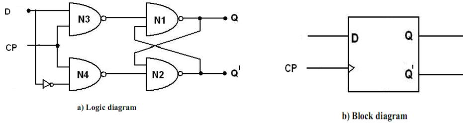
When the clock is low both the NAND gates (N1 and N2) are disabled and Q retains its last value. When clock is high both the gates are enabled and the input value at D is transferred to its output Q. D flip-flop is also called -Data flip-flop.
