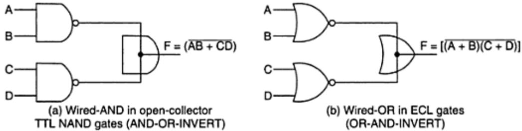
Similarly NOR outputs of ECL gates can be tied together to form Wired NOR function.
