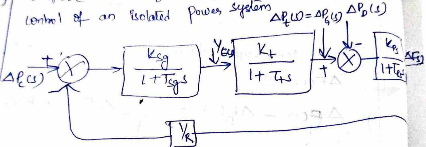
Block diagram model of load-frequency control
