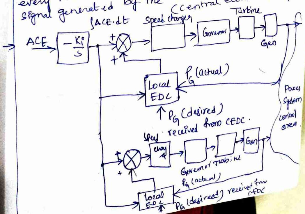
The above schematic diagram of both these units for two typical units of a control area.
