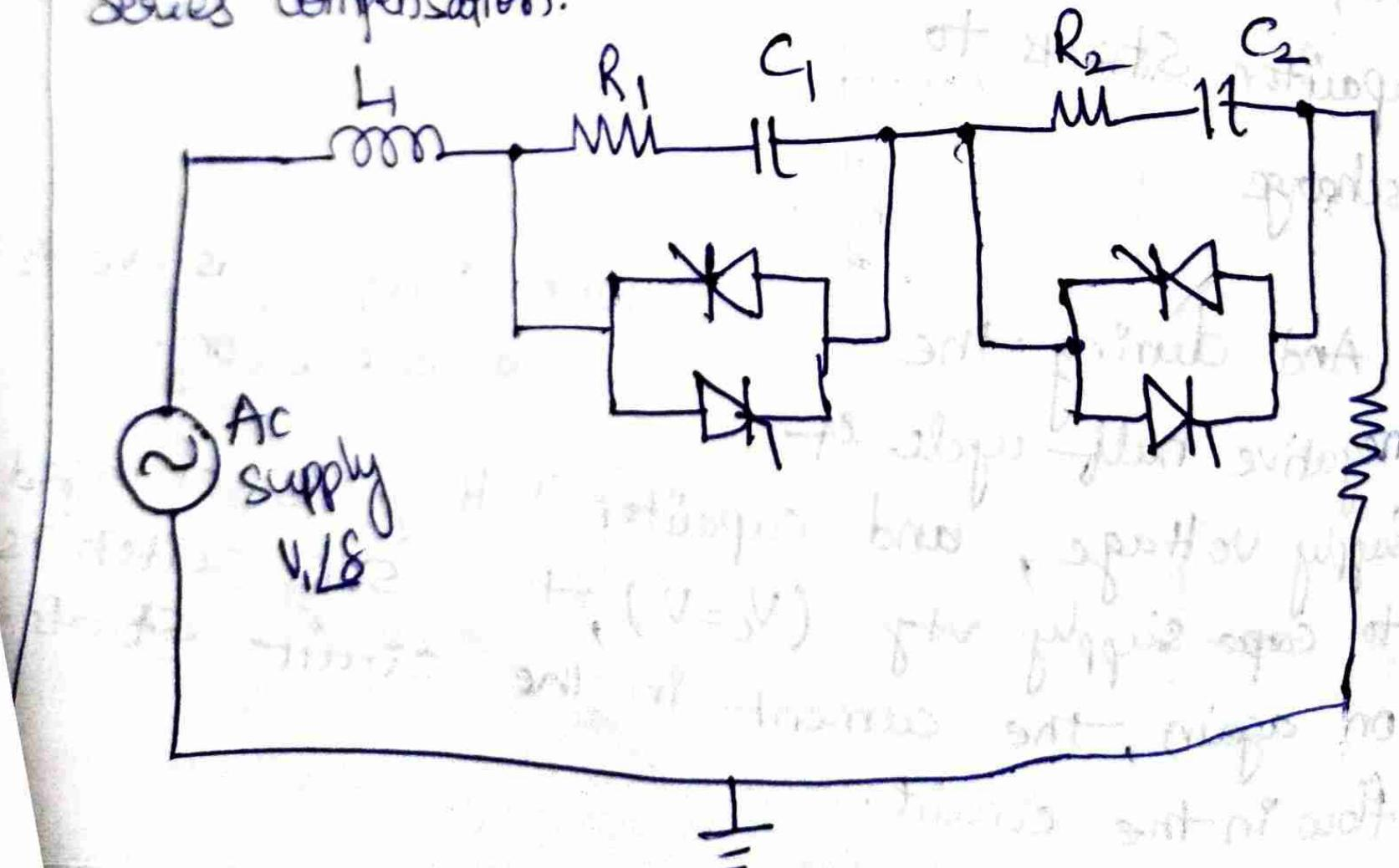
to accomplish this, each capacitor bank is controlled by a thyristor bypass switch or valve.
