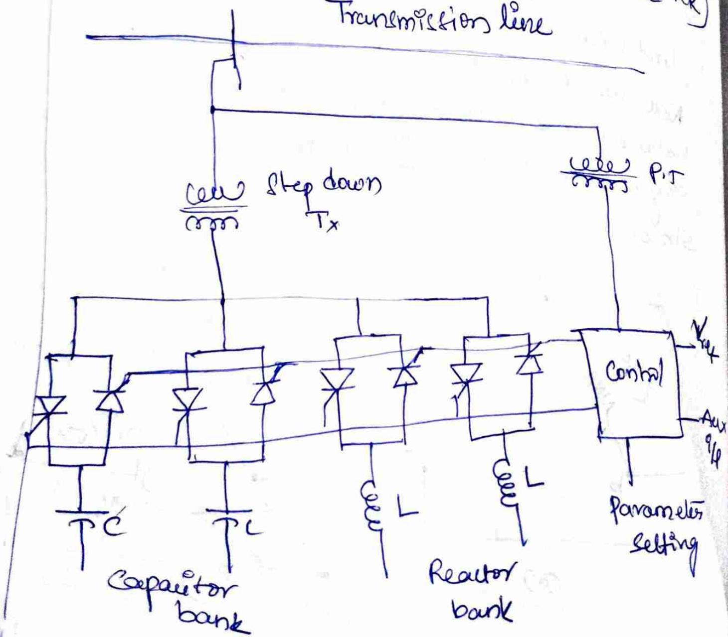
A shunt connected static VAR compensator, composed of TSCs and TCRs. With proper co-ordination of the capacitor switching and reactor control, the VAR output can be varied continuously.
