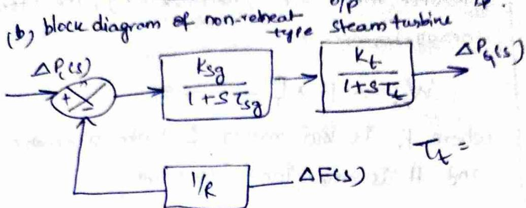
(c) T/F representation of speed control mechanism of a general generator with a non-reheat type steam turbine.
