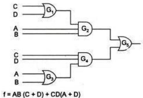
The C input to the OR gate must go through 3 levels of logic before reaching the output where as C input to the AND gate must only go through two levels, can result critical timing problem called *Logic Race*.
