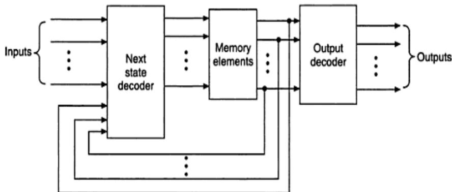
Figure: moore circuit model with an output decoder
