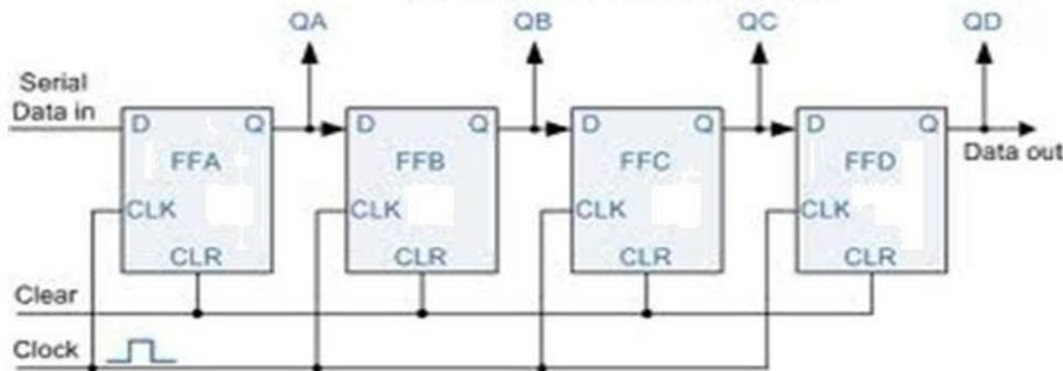
In this type of register, the data bits are entered into the register serially, but the data stored in the register is shifted out in parallel form.
