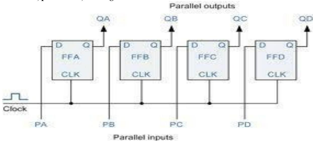
In a parallel-in, parallel-out shift register, the data is entered into the register in parallel form, and also the data is taken out of the register in parallel form. Data is applied to the D input terminals of the FF's. When a clock pulse is applied, at the positive going edge of the pulse, the D inputs are shifted into the Q outputs of the FFs. The register now stores the data. The stored data is available instantaneously for shifting out in parallel form.
