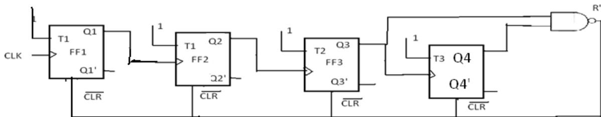
The count table and the K-Map for reset are shown in fig. from the K-Map  $R=Q4Q2$ . So, feedback is provided from second and fourth FFs. For active-HIGH reset,  $Q4Q2$  is applied to the clear terminal. For active-LOW reset  $\overline{Q4Q2}$  is connected to the clear terminal of all flip-flops.
