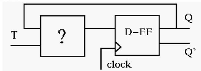
We need to design the circuit to generate the triggering signal D as a function of T and Q:
