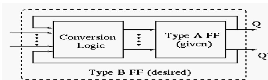
The key here is to use the excitation table, which shows the necessary triggering signal (S,R,J,K, D and T) for a desired flip-flop state transition :
