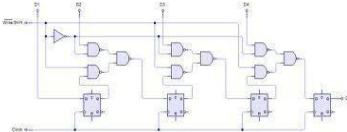
For a parallel-in, serial out, shift register, the data bits are entered simultaneously into their respective stages on parallel lines, rather than on a bit-by-bit basis on one line as with serial data bits are transferred out of the register serially. On a bit-by-bit basis over a single line.
