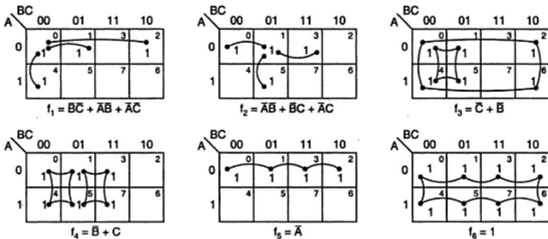
$f_3$  is read as  $\bar{C} + \bar{B}$ , because in the 4-square formed by  $m_0, m_2, m_6$ , and  $m_4$ , the variable A and B are changing, whereas the variable C remains constant as a 0. So it is read as  $\bar{C}$ . In the 4-square formed by  $m_0, m_1, m_4, m_5$ , A and C are changing but B remains constant as a 0. So it is read as  $\bar{B}$ . So, the resultant expression for  $f_3$  is the sum of these two, i.e.,  $\bar{C} + \bar{B}$ .
