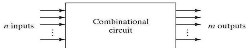
Fig. Block Diagram of Combinational Circuit
