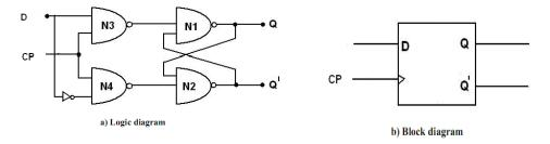
When the clock is low both the NAND gates (N1 and N2) are disabled and Q retains its last value. When clock is high both the gates are enabled and the input value at D is transferred to its output Q. D flip-flop is also called -Data flip-flop||.
