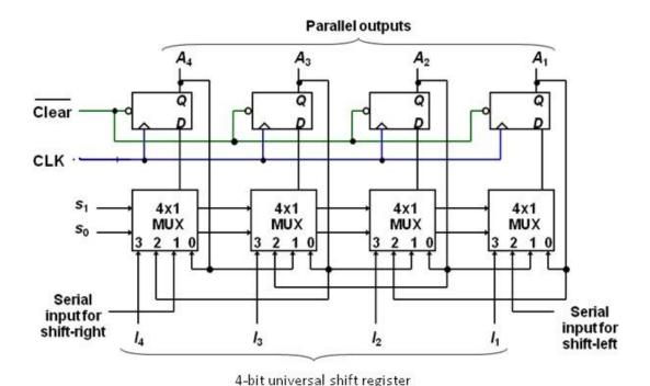
Figure: logic diagram 4-bit universal shift register
