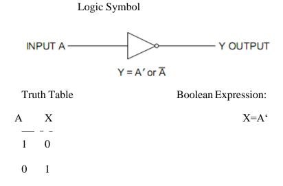
Logic circuits of any complexity can be realized using only AND, OR, NOT gates. Using these 3 called AND-OR-INVERT i.e, AOI Logic circuits.
