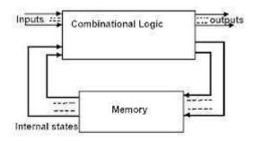
Figure 1: Asynchronous Sequential Circuit
