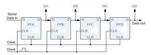
In this type of register, the data bits are entered into the register serially, but the data stored in the register is shifted out in parallel form.
