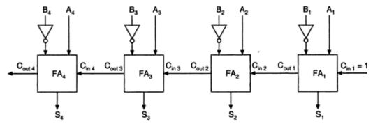
Logic diagram of a 4-bit parallel subtractor.
