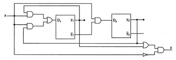
Fig: logic diagram of a mealy model
