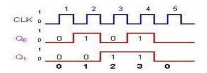
Two-bit ripple down-counter using negative edge triggered flip flop:
