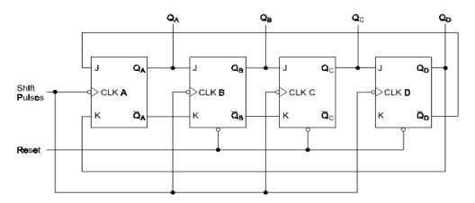
Figure: Johnson counter with JK flip-flops
