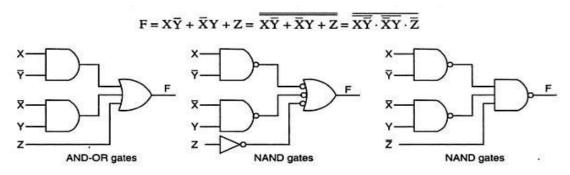
Two –level implementation using AND-OR and NAND logic
