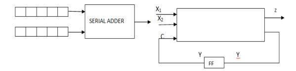
Figure: block diagram of serial binary adder
