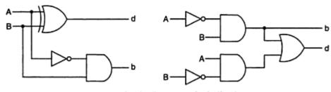
Logic diagrams of a half-subtractor.
