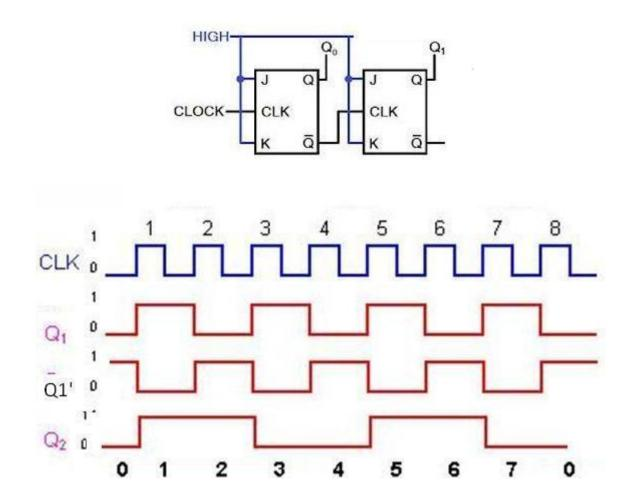
A 2-bit down-counter counts in the order 0,3,2,1,0,1.....,i.e, 00,11,10,01,00,11....,etc. the above fig. shows ripple down counter, using negative edge triggered J-K FFs and its timing diagram.
