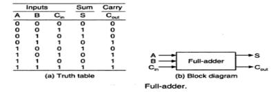
From the truth table, a circuit that will produce the correct sum and carry bits in response to every possible combination of A,B and C<sub>in</sub> is described by
