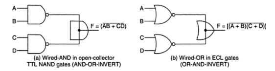
Similarly NOR outputs of ECL gates can be tied together to form Wired NOR function.
