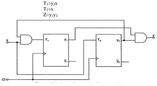
The characteristic equation of a T-flip-flop is
