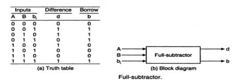
From the truth table, a circuit that will produce the correct difference and borrow bits in response to every possible combinations of A,B and  $b_i$  is
