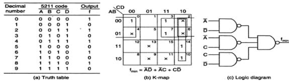
Truth table, K-map and logic diagram for the SOP circuit.
