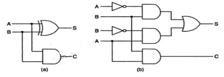
Logic diagrams of half-adder
