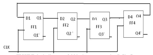
FIGURE: logic diagram of 4-bit ring counter using D flip-flops
