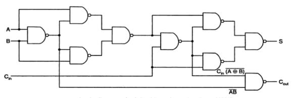
Logic diagram of a full-adder using only 2-input NAND gates.
