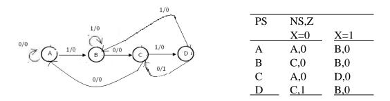
Figure: state diagram and state table of sequence detector
