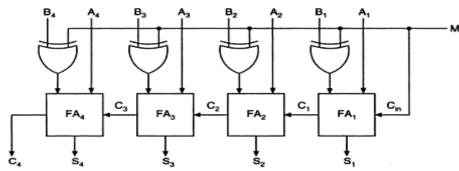
Logic diagram of a 4-bit binary adder-subtractor.
