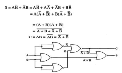
Logic diagram of a half-adder using only 2-input NOR gates.
