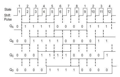
Figure: timing diagram
