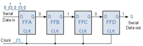
When serial data is transferred into a register, each new bit is clocked into the first FF at the positive going edge of each clock pulse. The bit that was previously stored by the first FF is transferred to the second FF. the bit that was stored by the Second FF is transferred to the third FF.
