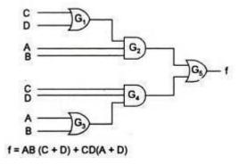
The C input to the OR gate must go through 3 levels of logic before reaching the output where as C input to the AND gate must only go through two levels, can result critical timing problem called *Logic Race*.
