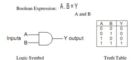
IC 7408 contains 4 two input AND gates
