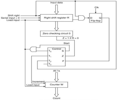
Datapath subsystem for weighing machine.
