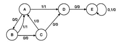
**Successor**: looking at the state diagram when present state is A and input is 1, the next state is D. this condition is specified as D is the successor of A. similarly we can say that A is the 1 successor of B, and C,D is the 11 successor of B and C, C is the 00 successor of A and D, D is the 000 successor of A,E, is the 10 successor of A or 0000 successor of A and so on.
