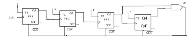
The count table and the K-Map for reset are shown in fig. from the K-Map R=Q4Q2. So, feedback is provided from second and fourth FFs. For active –HIGH reset, Q4Q2 is applied to the clear terminal. For active-LOW reset 4 2 is connected isof all Flip=flops.
