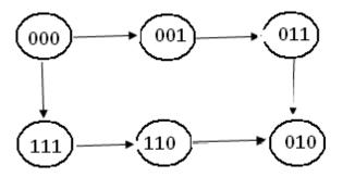
**Step3:** type of flip-flop and the excitation table: T flip-flops are selected and the excitation table of the mod-6 gray code counter using T-flip-flops is written as shown in fig.
