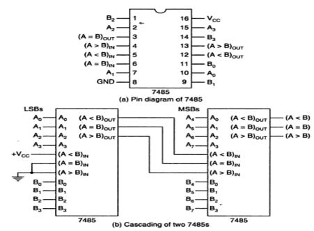
Pin diagram and cascading of 7485 4-bit comparators.
