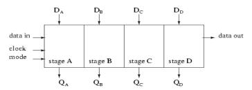
Parallel-in, parallel-out shift register with 4-stages
