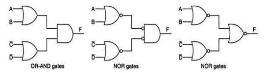
Two –level implementation using OR-AND and NOR logic
