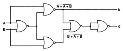
Logic diagram of a half-subtractor using only 2-input NOR gates.
