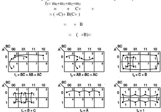
$f_3$  is read as + , because in the 4-square formed by m0,m2,m6, and m4, the variable A and B are changing , where as the variable C remains constant as a 0. So it is read as . In the 4-square formed by  $m_0$ , m1, m4,  $m_5$ , A and C are changing but B remains constant as a 0. So it is read as . So, the resultant expression for  $f_3$  is the sum of these two, i.e., + .
