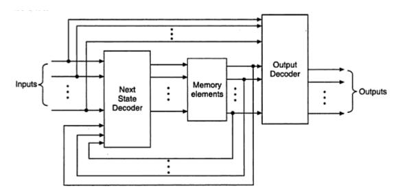
**Moore model:** when the output of the sequential circuit depends up only on the present state of the flip-flop, the sequential circuit is referred as to as the Moore circuit or the Moore machine.
