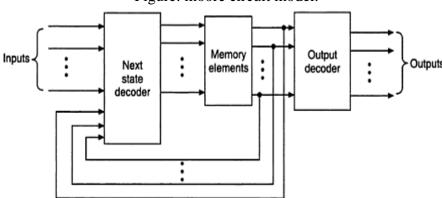
Figure: moore circuit model with an output decoder
