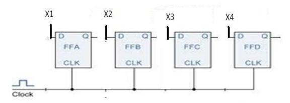
Figure: logic diagram of 4-bit buffer register
