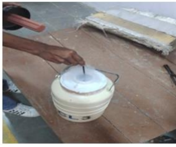
FIGURE 6. Keeping specimen in cryo-can
