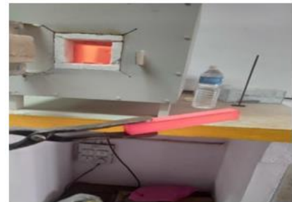
FIGURE 4. Specimen with austenizing Process
