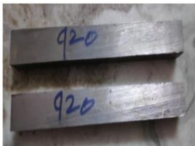
FIGURE 2. Specimen with austenizing process
