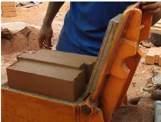
Fig 3. Making of Interlocking Moulded bricks.
