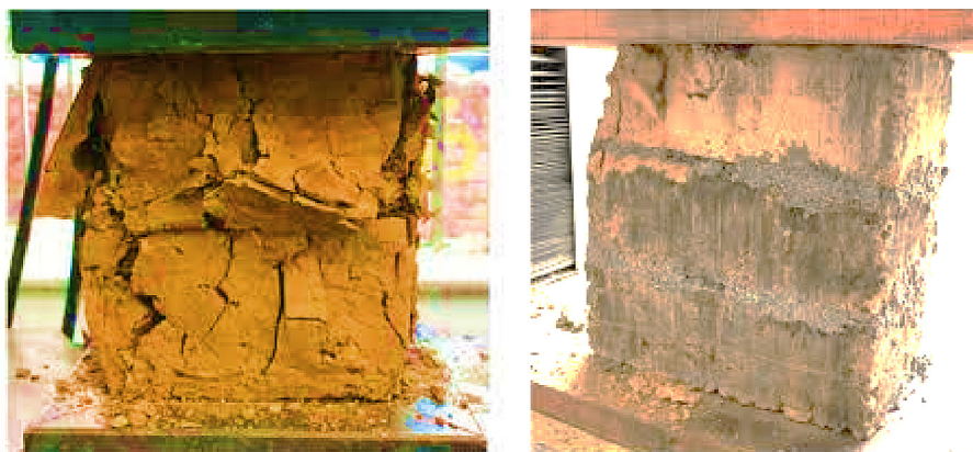
Fig. 8. Failure pattern for interlocking bricks under compression.
