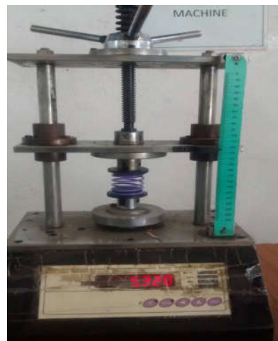
Fig.11 Set up for the experimental determination of spring stiffness
