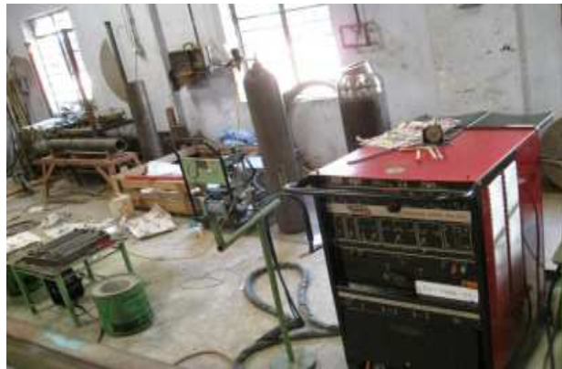
Figure 3: Lincoln Electrical Square Wave TIG 355 M/C
