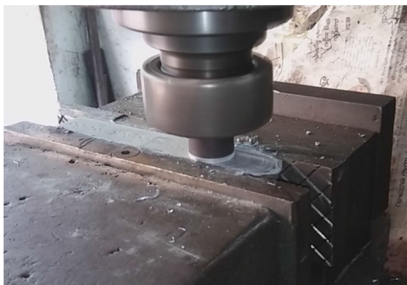
Fig. 3 Experimental setup for friction stir processing of Al-7075/SiC surface composite
