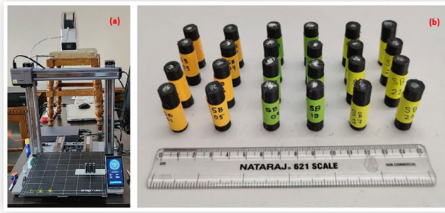
FIGURE 1 (a) FDM printer (b) Printed test samples
