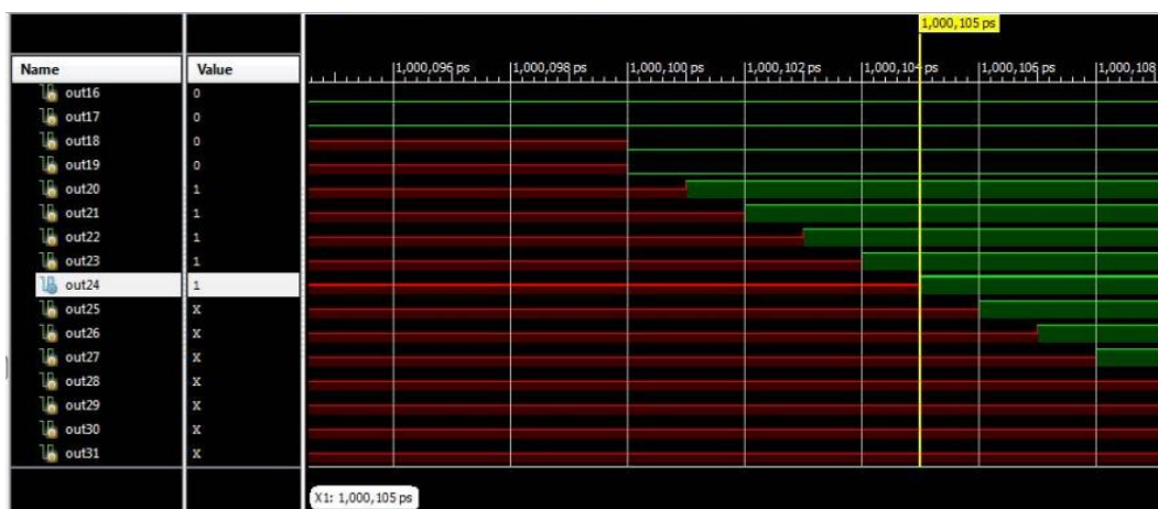
Figure 10: Simulation output wave for 32-different phase generator
