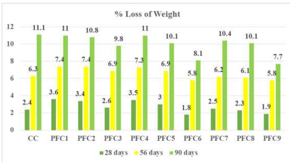
Figure 3 Percentage Loss of Weight- Acid Attack
