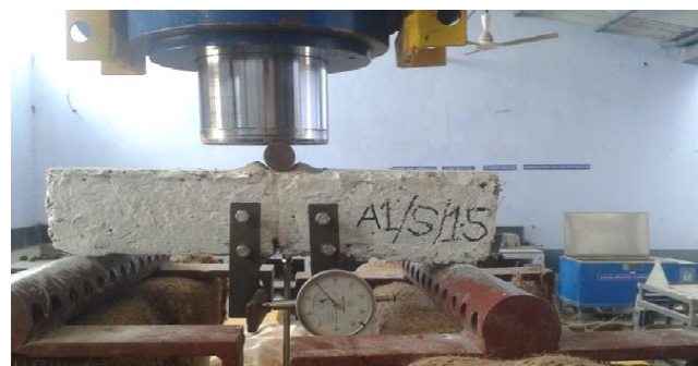
Fig. 4. BEAMS BEFORE TEST (A)
