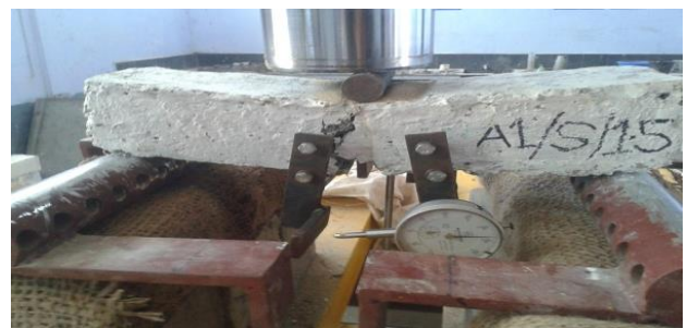
Fig. 5. BEAMS AFTER TEST(A)
