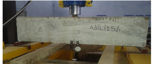
Fig. 2. Loading Frame Test Setup Used for Testing of Beams
