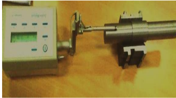
FIGURE 3. Photographic View Of Stylus During Surface Roughness Measurement
