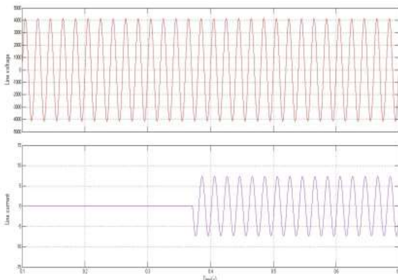
Figure 9 Shunt-CMI line voltage V_{Pab} and line current \vec{I}_{La} in case1 to case2.
