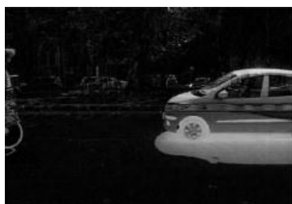
Fig 1: Result of Frame differencing being performed on (a) Frame X and (b) Frame Y with background frame.
