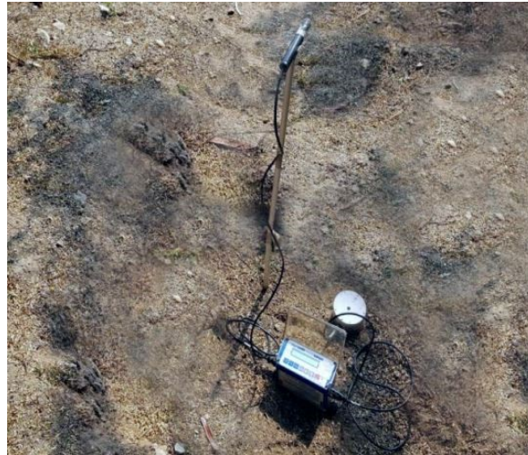
Figure 8. Data collection using Minimate blaster
