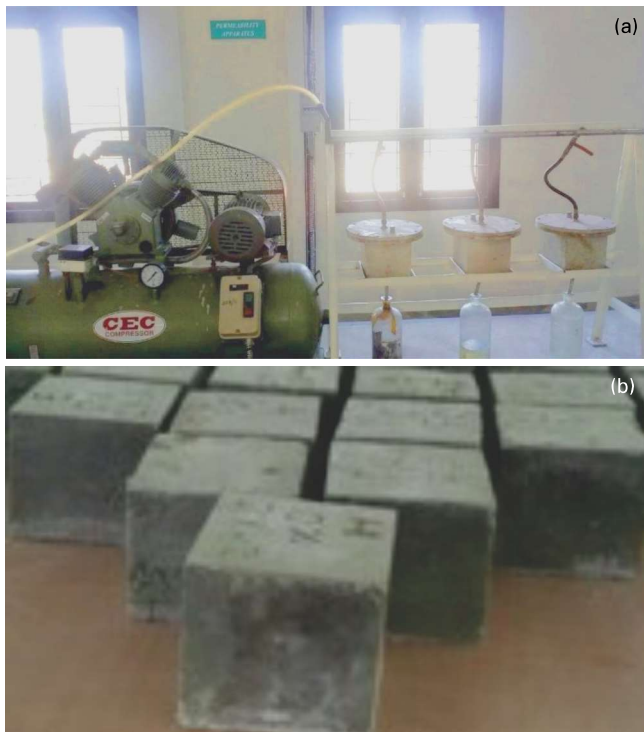
Figure 5. (a) Experimental setup for permeability test and (b) cubes casted for the test
