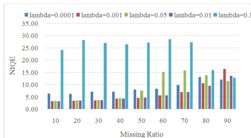
Fig. 5 (c) NIQE of Parrot image recovered from different missing ratios and different Lambda values
