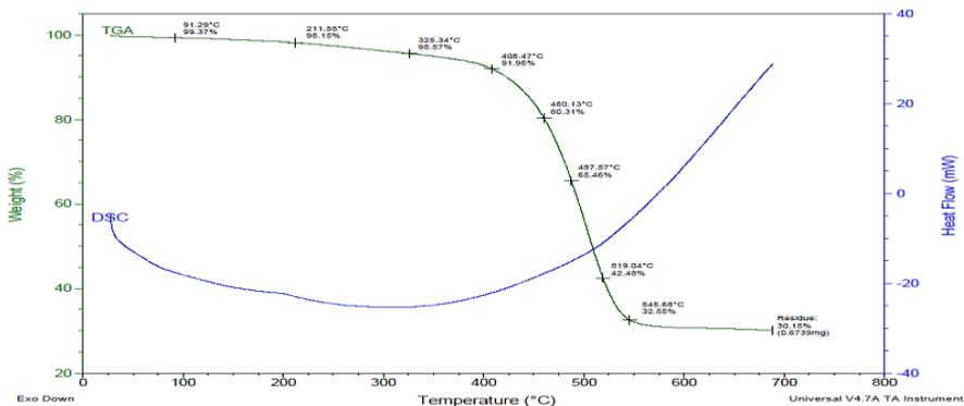
**Fig. 5.** DSC and TGA characteristic curve for synthetic rubber with 2% Alumina
