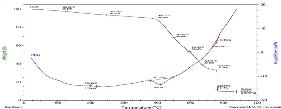
**Fig. 4.** DSC and TGA characteristic curve for rubber with 3% Titanium di Oxide
