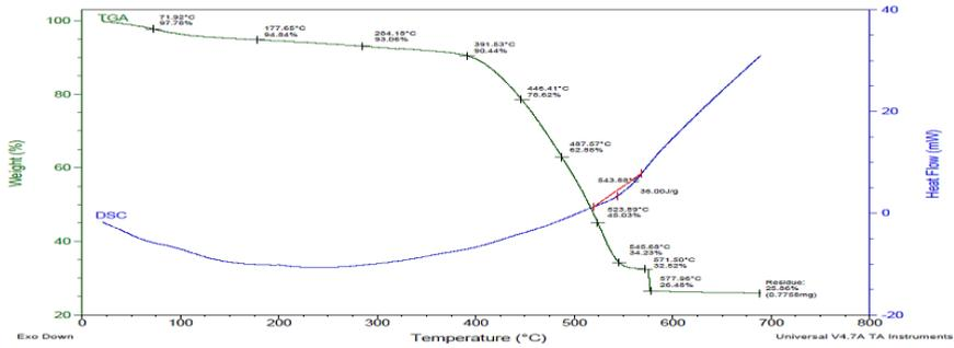
**Fig 6.** DSC and TGA characteristic curve for rubber with 3% Barium Titanate
