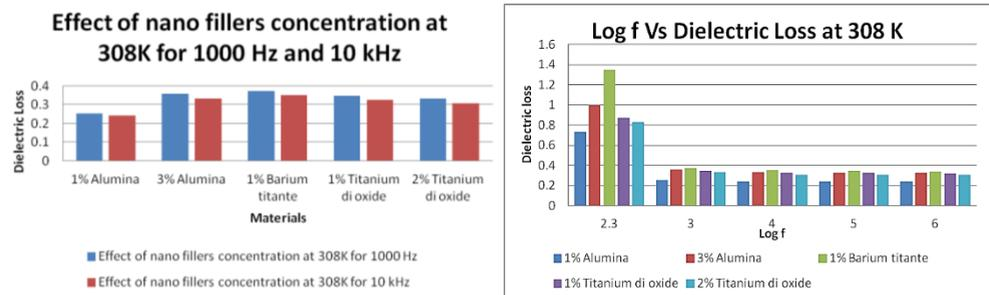
**Fig. 11.** Effect of Nano Fillers At 308K for 1000Hz and 10kHz & Log f Vs Dielectric loss at 308 K
