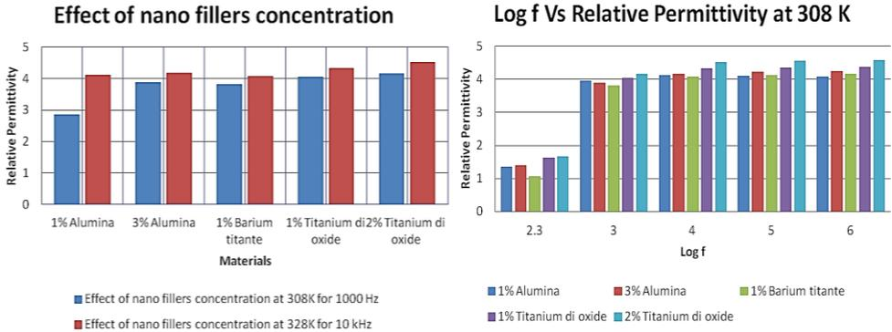
**Fig. 10.** Effect of nano filler concentration at 308K for 1000HZ and 328K for 10kHz & Log F Vs Relative Permittivity for Various Nano-Composites
