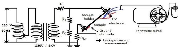
**Fig. 1.** Inclined Plane Tracking and Erosion Test Setu.
