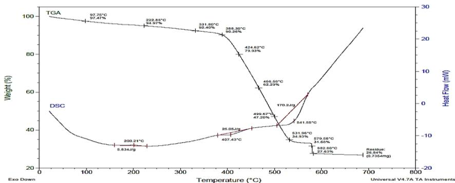
**Fig. 3.** DSC and TGA characteristic curve for synthetic rubber with 3% Alumina
