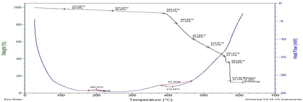
**Fig. 7.** DSC and TGA characteristic curve for rubber with 2% Titanium di Oxide
