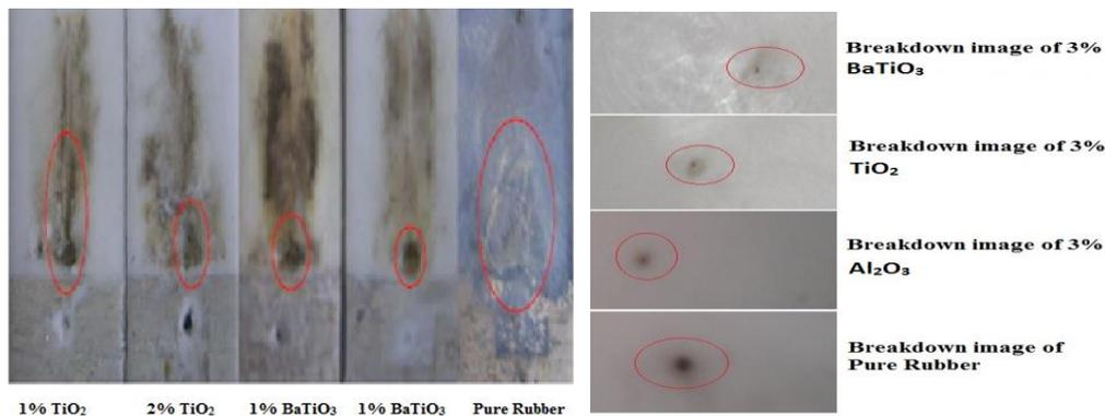
**Fig. 9.** Tracking images for various components & Breakdown images for various components
