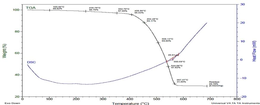
Fig. 2. DSC and TGA characteristic curve for synthetic rubber
