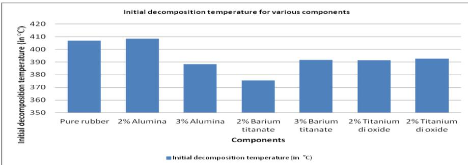
**Fig. 8.** Initial decomposition temperature for various components
