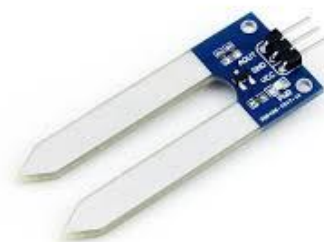
Figure (3) Humidity Sensor
