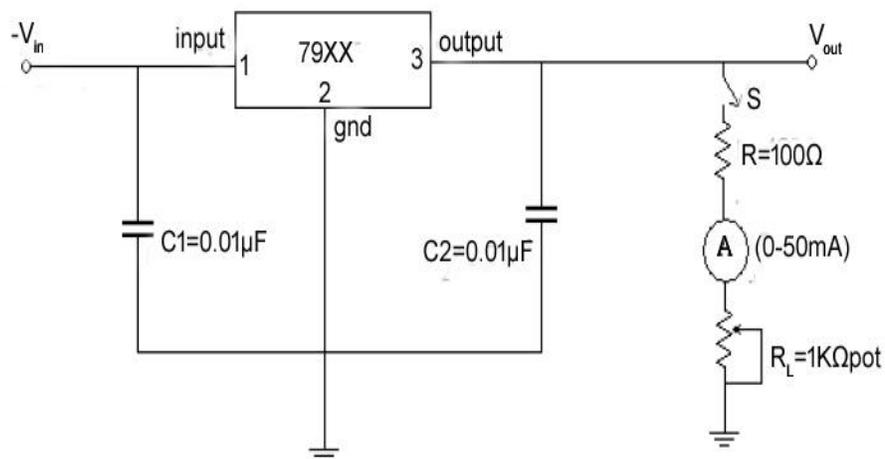
**Figure: 3. Negative Voltage Regulator**
