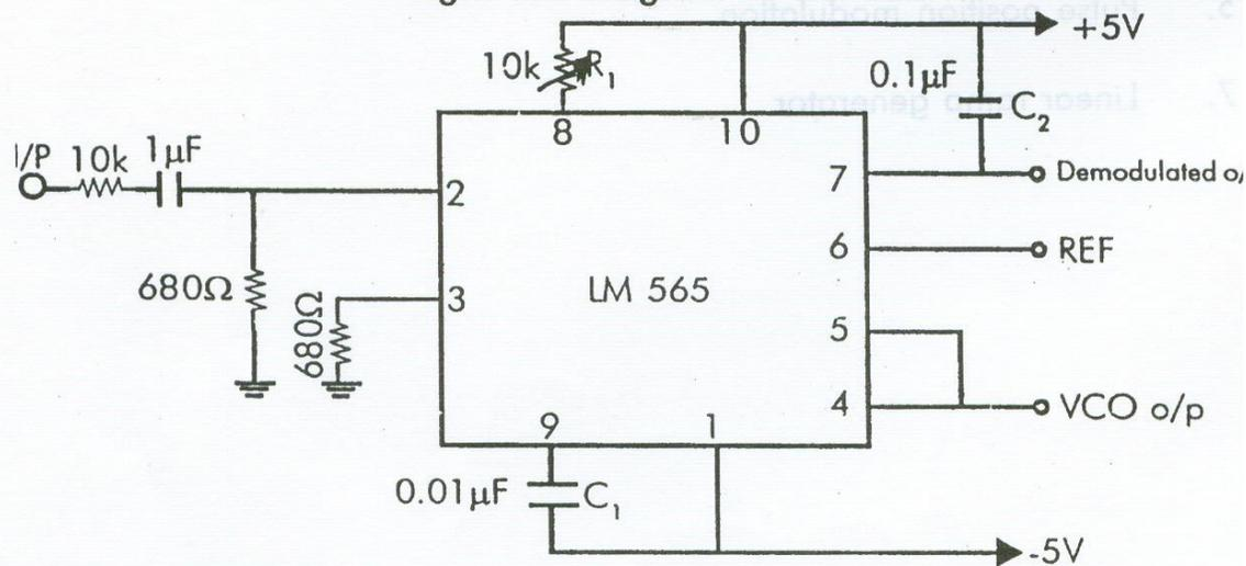
Fig.2 Circuit Diagram of LM 565
