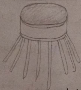
Top-5-style package Tab locates pin 8
