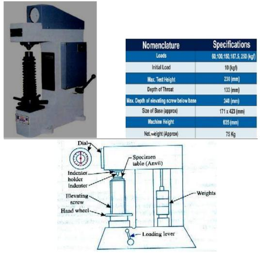
**THEORY:** The hardness of a material is resistance to penetration under a localized pressure or resistance to abrasion. Hardness tests provide an accurate, rapid and economical way of determining the resistance of materials to deformation. There are three general types of hardness measurements depending upon the manner in which the test is conducted:
