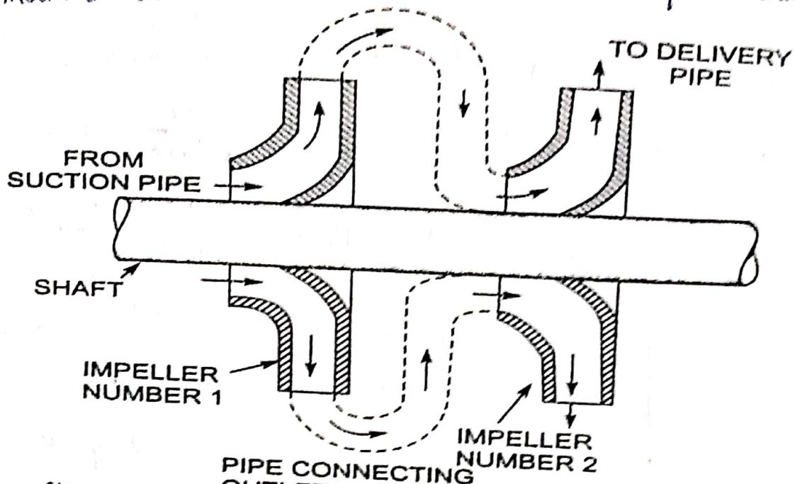
The water enters the 1st impeller at the inlet of the 1st impeller.
