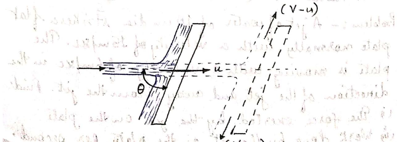
Let a jet of water strikes an inclined plate, which is moving with a uniform velocity in the direction of the jet as shown in the figure.
