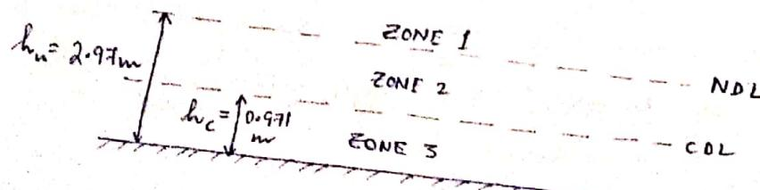
From the figure, it is evident that the depth of zone 1 is 2.97 m and the depth of zone 3 is 0.972 m.
