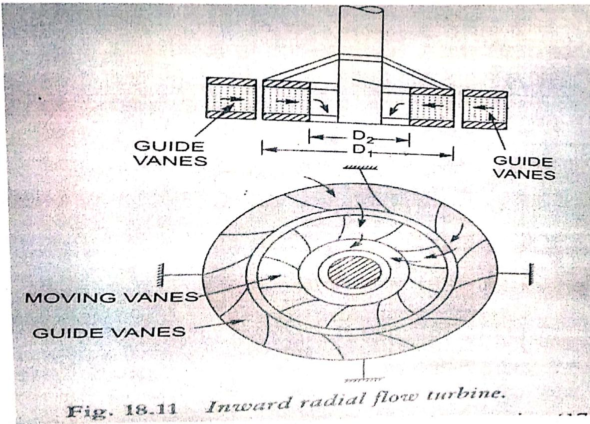
Fig. 18.11 Inward radial flow turbine.
