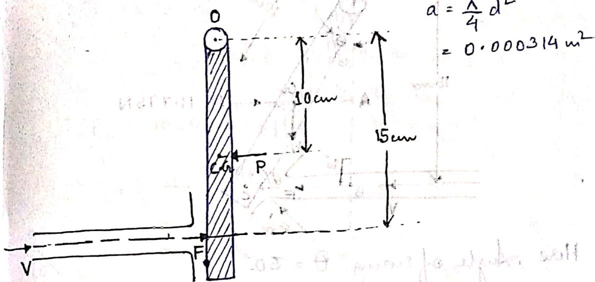
In this case, since an attempt is made to keep the plate in vertical position by applying a force  $P$  at the C.G. of the plate, the plate eventually becomes stationary.
