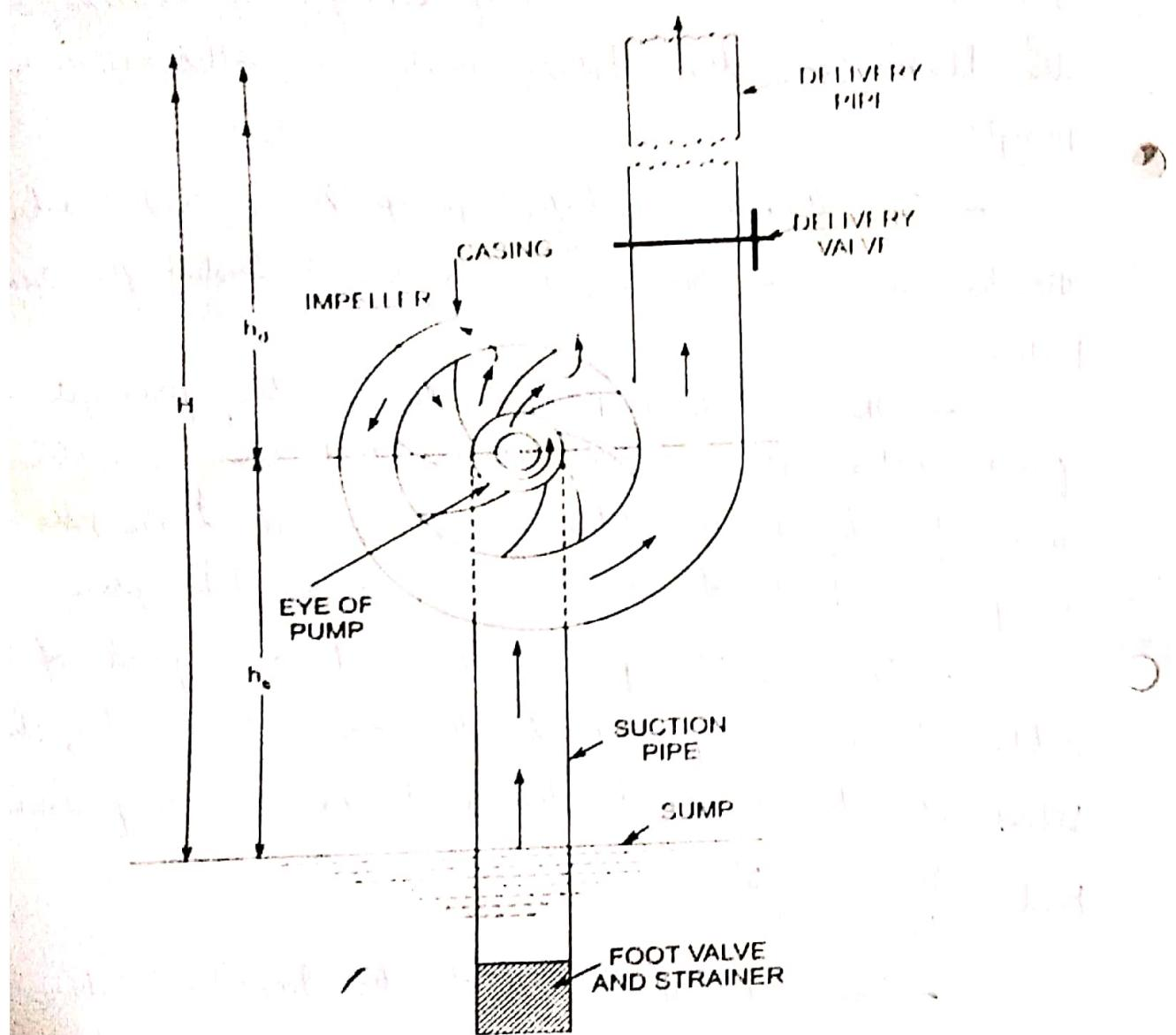
Fig-1 : Main Parts of a Centrifugal Pump
