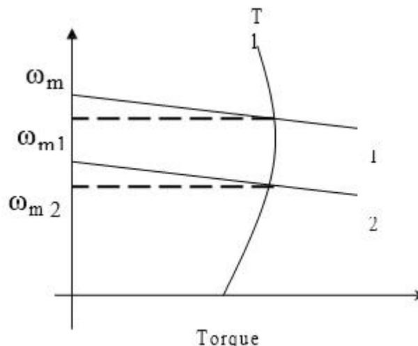
Acceleration and Deceleration modes are transient modes. Drive operates in acceleration mode whenever an increase in its speed is required. For this motor speed torque curve must be changed so that motor torque exceeds the load torque. Time taken for a given change in speed depends on inertia of motor load system and the amount by which motor torque exceeds the load torque.
