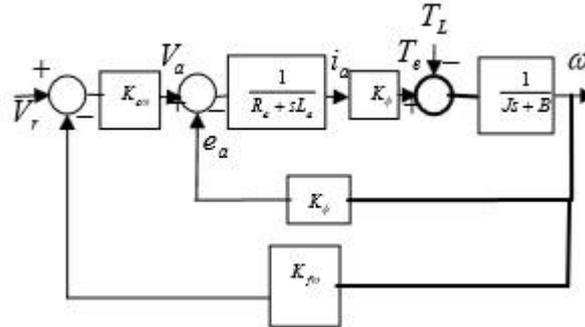
Block Diagram of the Closed Loop Speed Control.
