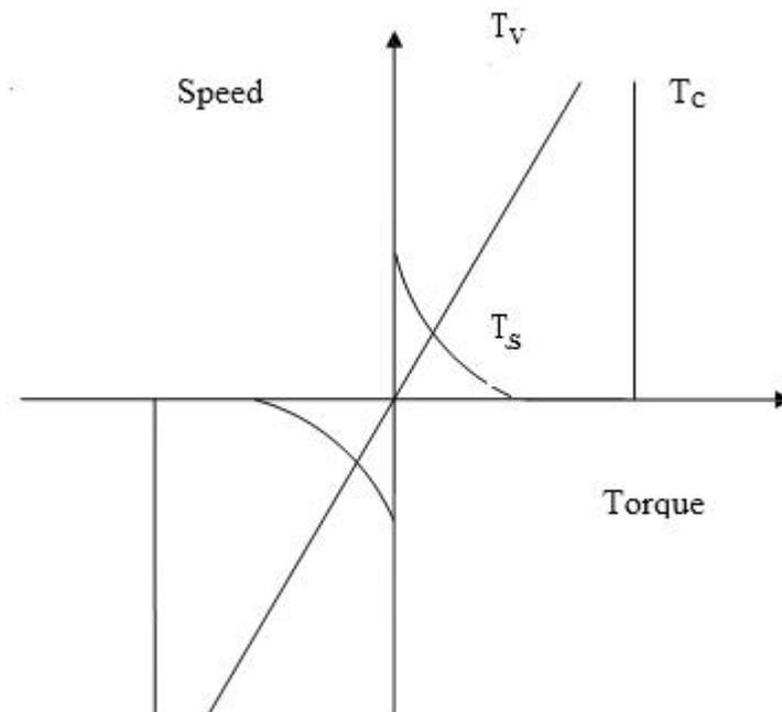
Component  $T_v$  varies linearly with speed is called VISCOUS friction and is given by
