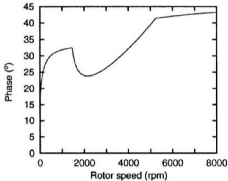
Angle between stator voltage and stator current  $\phi$ .
