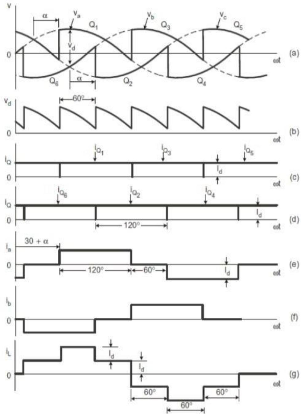
Fig 2.14 Three-phase thyristor bridge waveforms in rectification mode ( $\alpha = 40^\circ$ )
