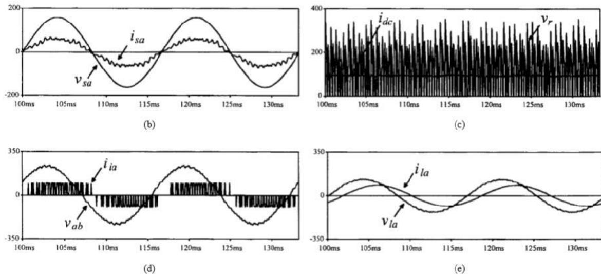
AC drive CSI based on a PWM front-end rectifier
