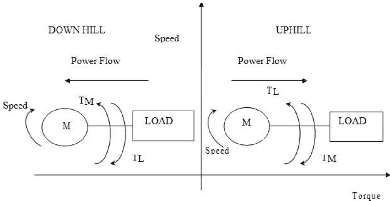
Now we consider that the same bus is traveling in down hill, the gravitational force doesn't change its direction but the load torque pushes the motor towards the bottom of the hill. The motor produces a torque in the reverse direction because the direction of the motor torque is always opposite to the direction of the load torque.
