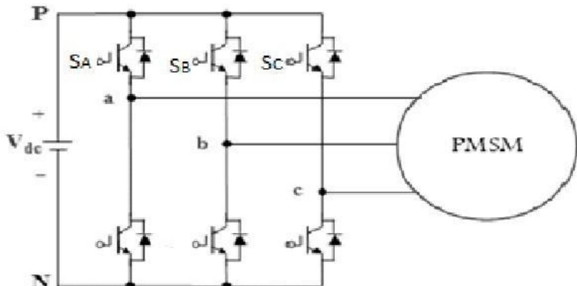
Diagram of a three phase inverter
