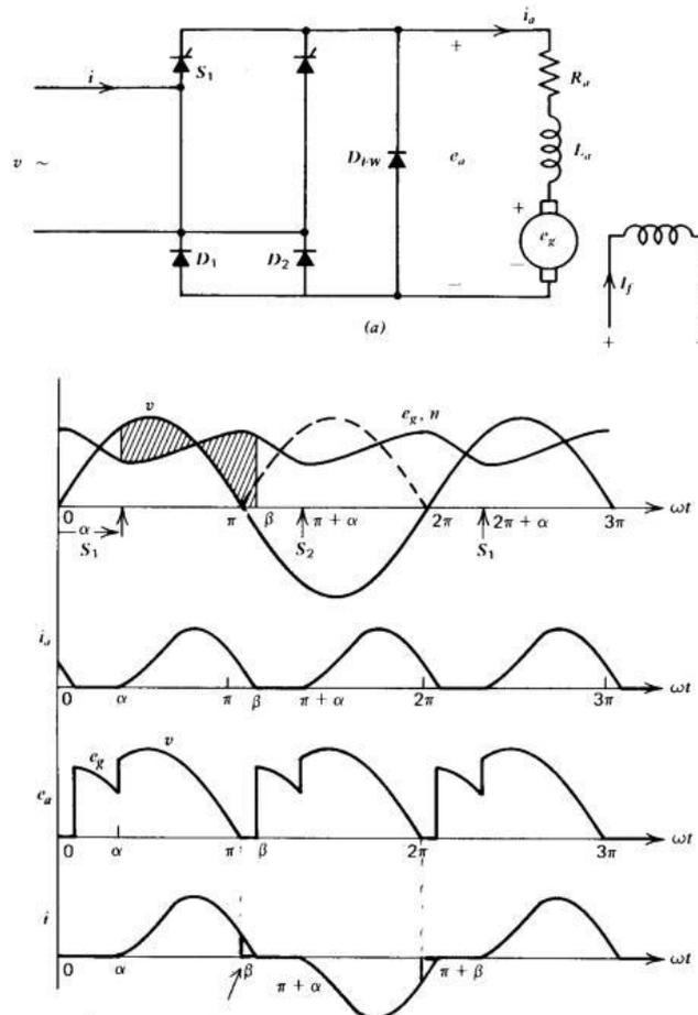
**Fig. 2.5** Effects of discontinuous motor current in semi-converter operation. (a) Power circuit. (b) Voltage and current waveforms.
