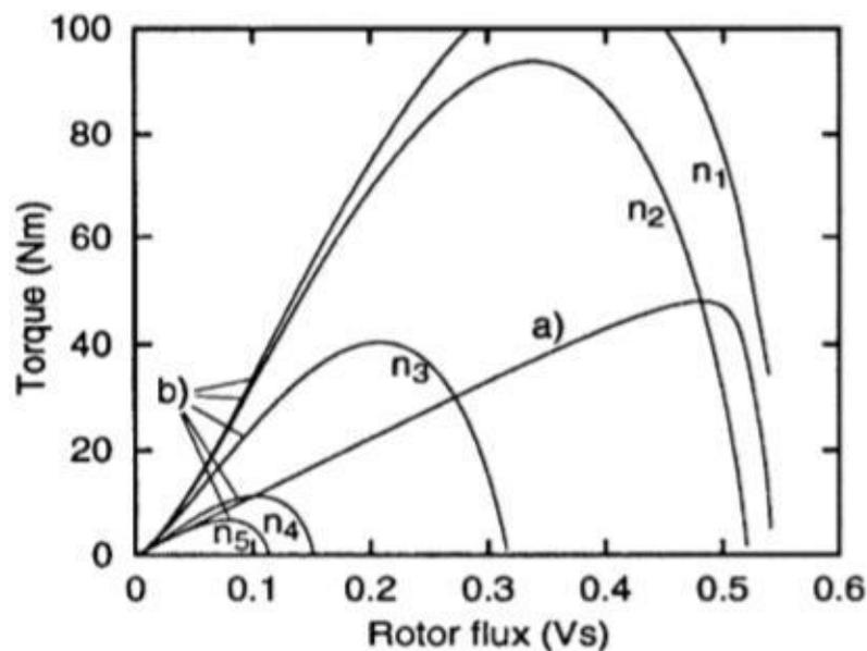
Lower flux weakening region: At medium speeds the maximum torque is indicated by the crossing of both limitation curves (e. g. curve a) and b) with 2500 rpm). The induction machine has to run with minimum current and maximum voltage.
