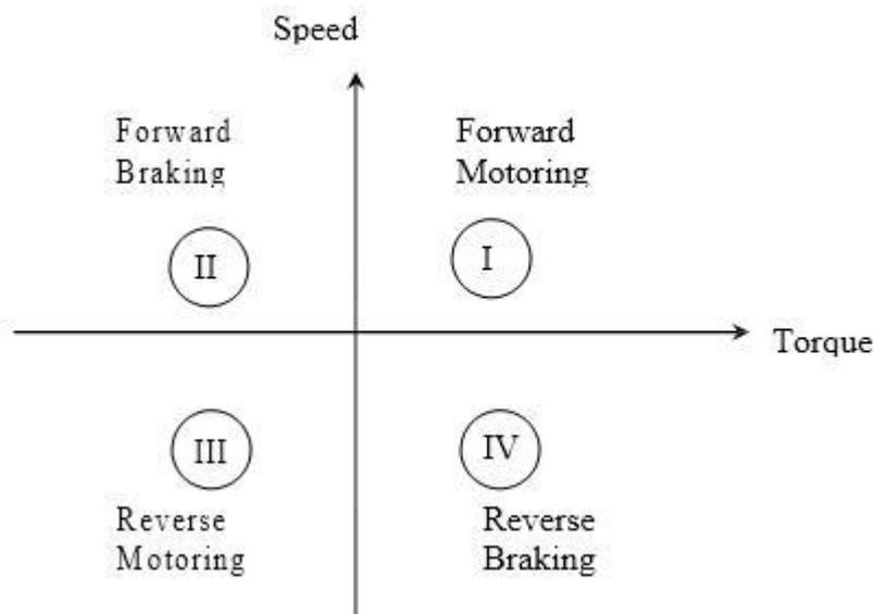
For better understanding of the above notations, let us consider operation of hoist in four quadrants as shown in the figure. Direction of motor and load torques and direction of speed are marked by arrows.
