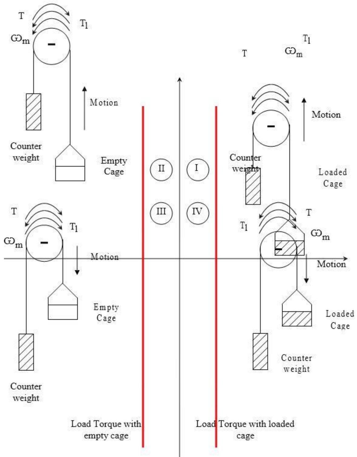
A hoist consists of a rope wound on a drum coupled to the motor shaft one end of the rope is tied to a cage which is used to transport man or material from one level to another level . Other end of the rope has a counter weight. Weight of the counter weight is chosen to be higher than the weight of empty cage but lower than of a fully loaded cage.
