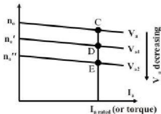
As flux remains constant, this method is suitable for constant torque loads. In a way armature voltage control method dissimilar to that of armature resistance control method except that the former
