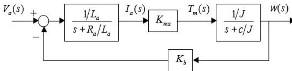
Block diagram reduction gives the transfer function from the input armature voltage to the resulting speed change.
