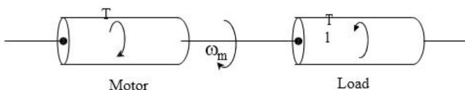
$J$  = Moment of inertia of motor load system referred to the motor shaft  $\text{kg} / \text{m}^2$
