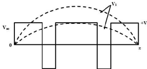
PWM principle to control output voltage.
