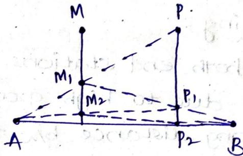
\* As shown in the above fig. Station A & B are not inter visible due to high level ground in b/w.
