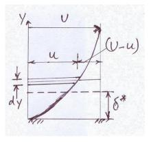
Fig. Displacement Thickness **Momentum thickness** □
