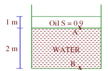
$p_A = \gamma_{a1} h_{oil}$ = (0.9 x 9.81) x 1  $p_A = 8.829 \text{ kPa}$  $p_B = \gamma_{oil} xh_{oil} + \gamma_{water} + h_{water}$  $p_A = 8.829 \text{ kPa} + 9.81 \text{ x } 2$  $p_B = 28.45 \text{ kPa}$
