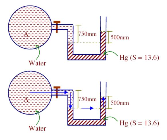
Let ' $h_A$ ' be the pressure head at 'A' in 'meters of water'.
