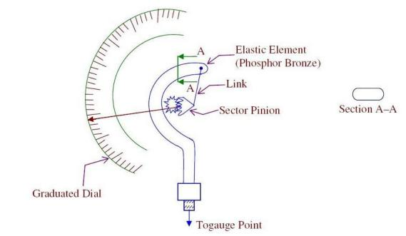
Mechanical gauge consists of an elastic element which deflects under the action of applied pressure and this deflection will move a pointer on a graduated dial leading to the measurement of pressure. Most popular pressure gauge used is Bordon pressure gauge.
