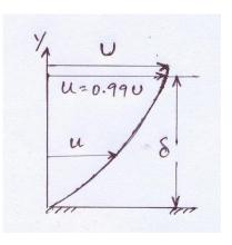
If the plate is smooth, the turbulent boundary layer consists of a thin layer adjacent to the boundary in which the flow is laminar. This thin layer is known as the laminar sub-layer.
