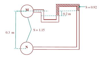
Let ' $h_M$ ' and ' $h_N$ ' be the pressure heads at M and N in m of water.
