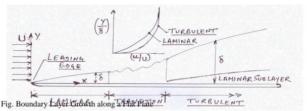
Up to a certain length along the plate from the leading edge, boundary layer thickness increases and the boundary layer exhibits the characteristics of a laminar flow irrespective of whether the incoming flow is laminar or turbulent. – This is known as laminar boundary layer. The thickness of the laminar boundary layer ( $\Box$ ) is given by ( $\Box$ ) = y (at (u/U) = 0.99) where u = local velocity.
