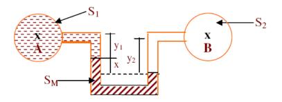
A differential U-tube manometer is used to measure pressure difference between any two points. It consists of a U-tube containing heavier manometric liquid, the two limbs of which are connected to the gauge points between which the pressure difference is required. U-tube differential manometers can also be used for gases. By writing the gauge equation for the system pressure difference can be determined.
