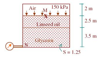
$P_{H} = 150 \text{ kPa}$  $h_{M} = \frac{150}{9.81}$  $h_{M} = 15.29 \text{ m of water}$
