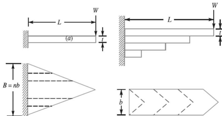
If a triangular plate is used as shown in Fig., the stress will be uniform throughout. If this triangular plate is cut into strips of uniform width and placed one below the other, as shown in Fig. to form a graduated or laminated leaf spring, then
