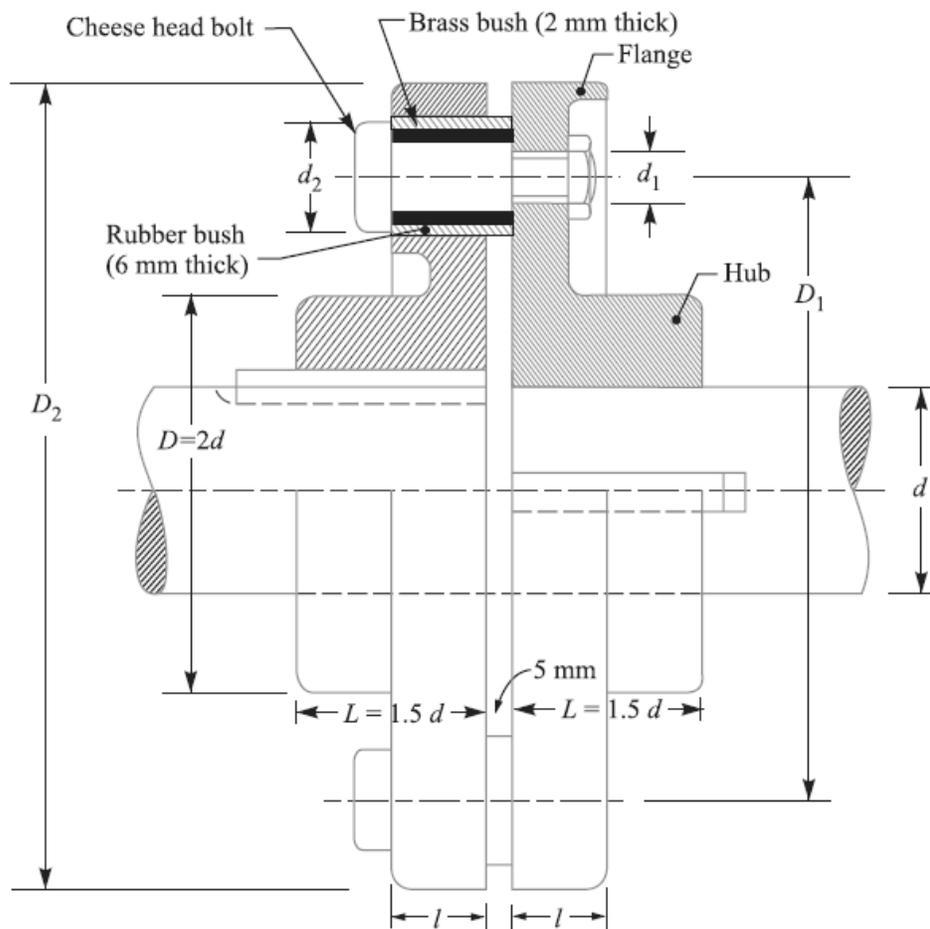
The rubber or leather bushes are used over the pins. The two halves of the coupling are dissimilar in construction. A clearance of 5 mm is left between the face of the two halves of the coupling. There is no rigid connection between them and the drive takes place through the medium of the compressible rubber or leather bushes.
