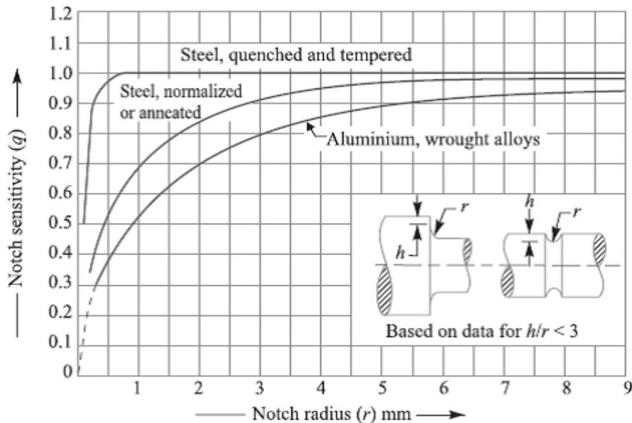
$$K_f = 1 + q (K_t - 1) \quad \dots[\text{For tensile or bending stress}]$$
