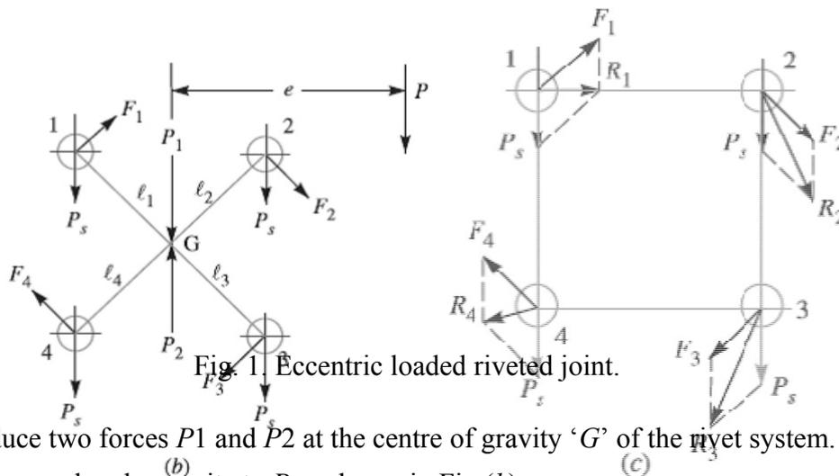
Fig. 1. Eccentric loaded riveted joint.
