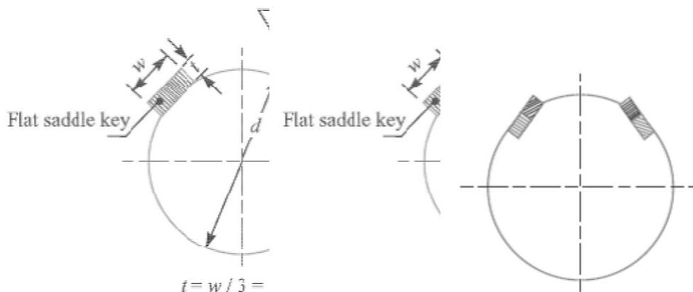
Fig. Flat saddle key and Tangent keys
