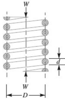
a) Axially loaded helical spring.
