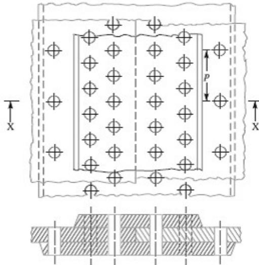
**Fig.1.** Triple riveted double strap (unequal) butt joint.
