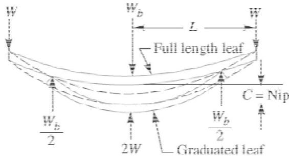
Consider that under maximum load conditions, the stress in all the leaves is equal. Then at maximum load, the total deflection of the graduated leaves will exceed the deflection of the full length leaves by an amount equal to the initial gap  $C$ . In other words,
