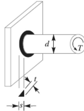
Fig. 1. Circular fillet weld subjected to torsion.
