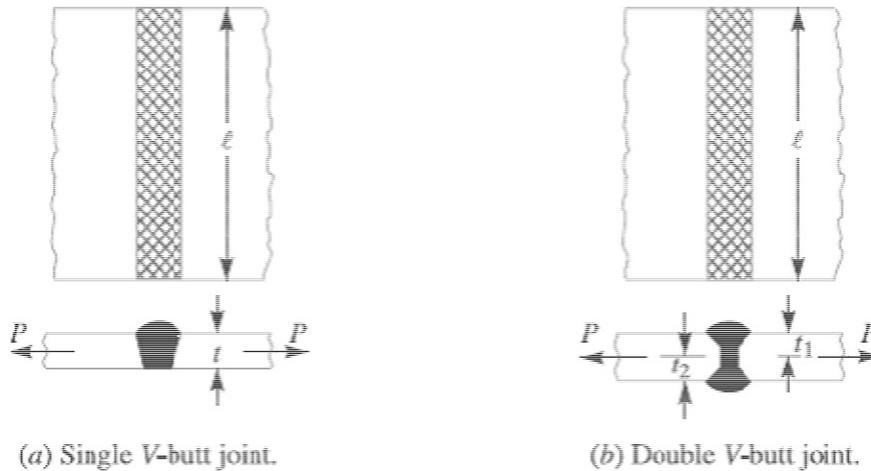
Fig.4. Butt Joints
