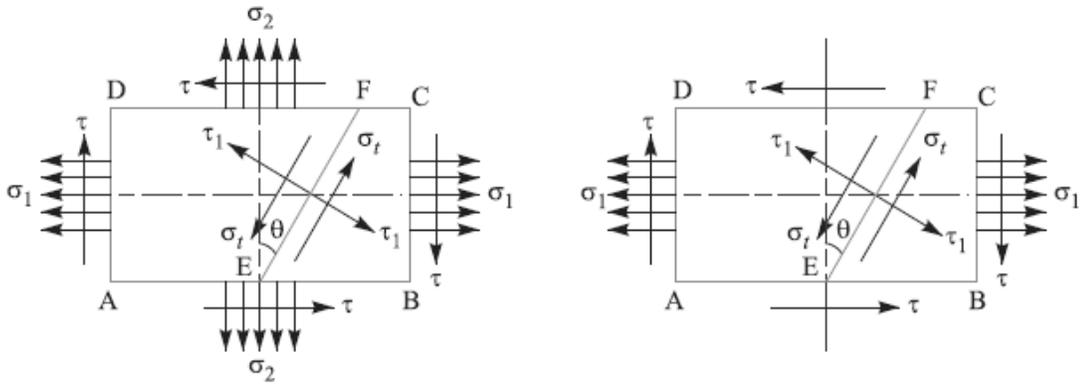
(a) Direct stress in two mutually perpendicular planes accompanied by simple shear stress.
