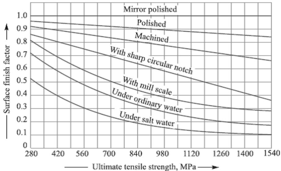
When the surface finish factor is known, then the endurance limit for the material of the machine member may be obtained by multiplying the endurance limit and the surface finish factor. We see that for a mirror polished material, the surface finish factor is unity. In other words, the endurance limit for mirror polished material is maximum and it goes on reducing due to surface condition.
