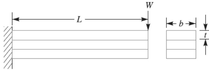
The above relations give the stress and deflection of a leaf spring of uniform cross section. The stress at such a spring is maximum at the support.
