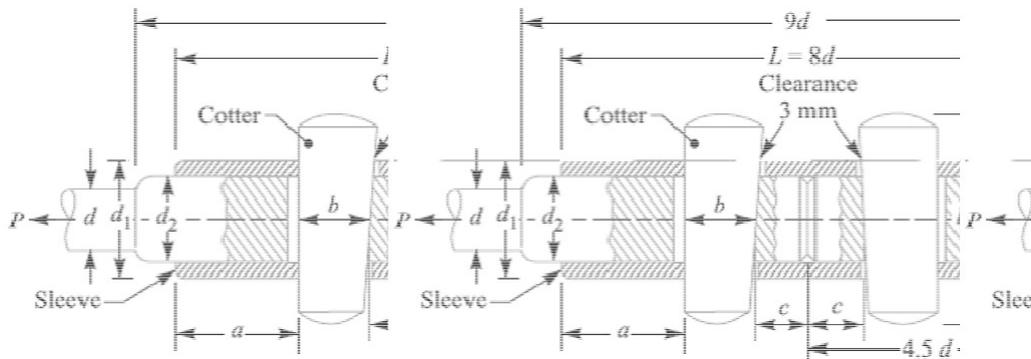
The various proportions for the sleeve and cotter joint in terms of the diameter of rod ( $d$ ) are as follows :
