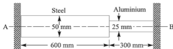
**Solution.** Given :  $t_1 = 37^\circ\text{C}$ ;  $t_2 = 20^\circ\text{C}$ ;  $E_s = 210\text{ GPa} = 210 \times 10^9\text{ N/m}^2$ ;  $E_a = 74\text{ GPa} = 74 \times 10^9\text{ N/m}^2$ ;  $\alpha_s = 11.7 \times 10^{-6} / ^\circ\text{C}$ ;  $\alpha_a = 23.4 \times 10^{-6} / ^\circ\text{C}$ ;  $d_s = 50\text{ mm} = 0.05\text{ m}$ ;  $d_a = 25\text{ mm} = 0.025\text{ m}$ ;  $l_s = 600\text{ mm} = 0.6\text{ m}$ ;  $l_a = 300\text{ mm} = 0.3\text{ m}$
