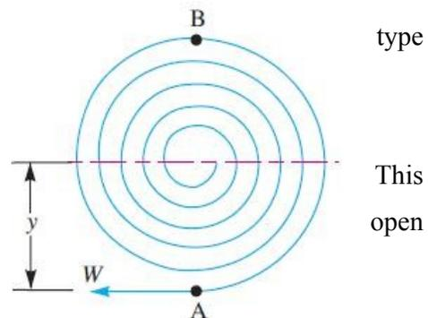
pinned or clamped. Since the radius of curvature of every spiral decreases when the spring is wound up, therefore the material of the spring is in a state of pure bending. Let  $W$  = Force applied at the outer end  $A$  of the spring,
