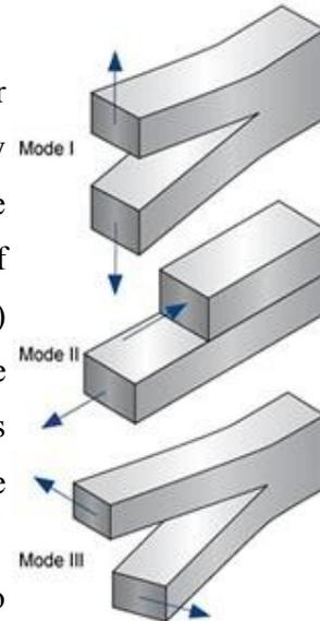
A parameter called the stress-intensity factor (K) is used to determine the fracture toughness of most materials. A Roman
