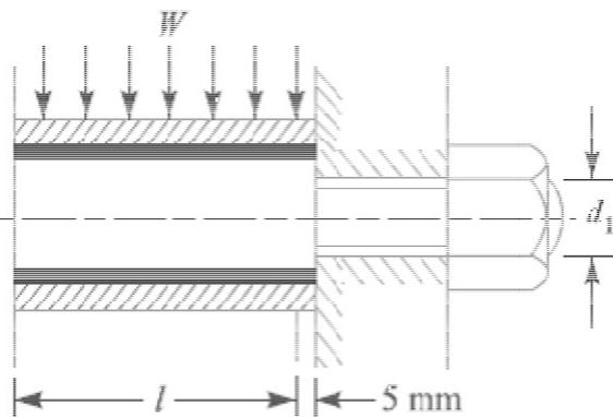
on the pin as shown in Fig. The bush portion of the pin acts as a cantilever beam of length  $l$ . Assuming a uniform distribution of the load  $W$  along the bush, the maximum bending moment on the pin,
