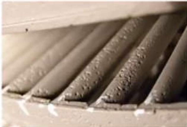
**If steam quality is less than 85% Erosion of turbine blade take place
