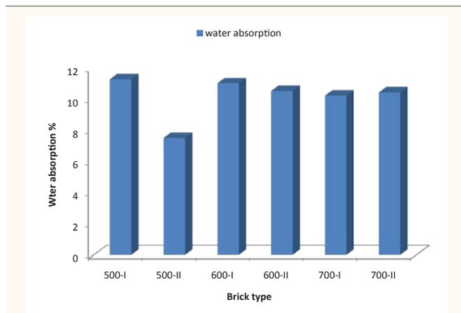
Figure 3 Water absorption test of the fired bricks.
