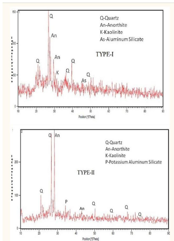
**Figure 5** XRD pattern of the fired brick.
