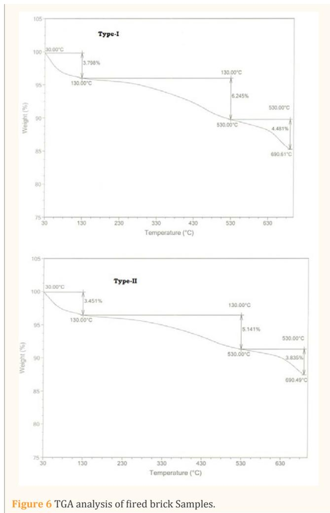
Figure 6 TGA analysis of fired brick Samples.
