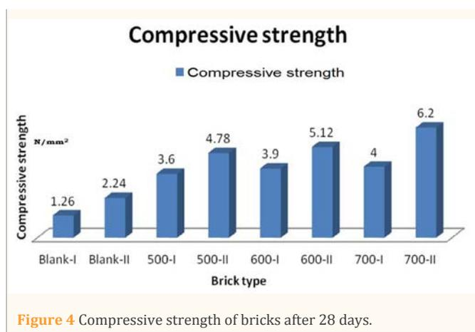
**Figure 4** Compressive strength of bricks after 28 days.
