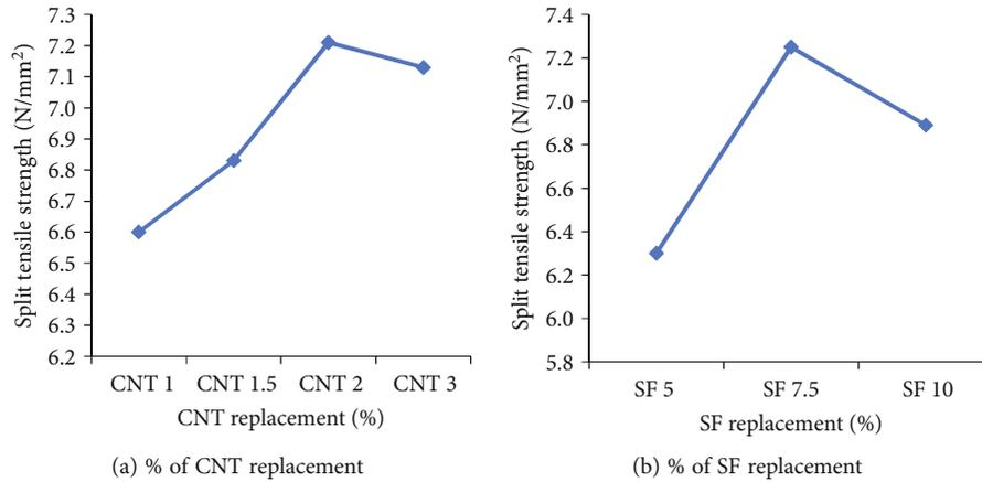
FIGURE 7: Split tensile strength variation at the 28<sup>th</sup> day.TABLE 9: Concrete flexural strength at the 28<sup>th</sup> day.
