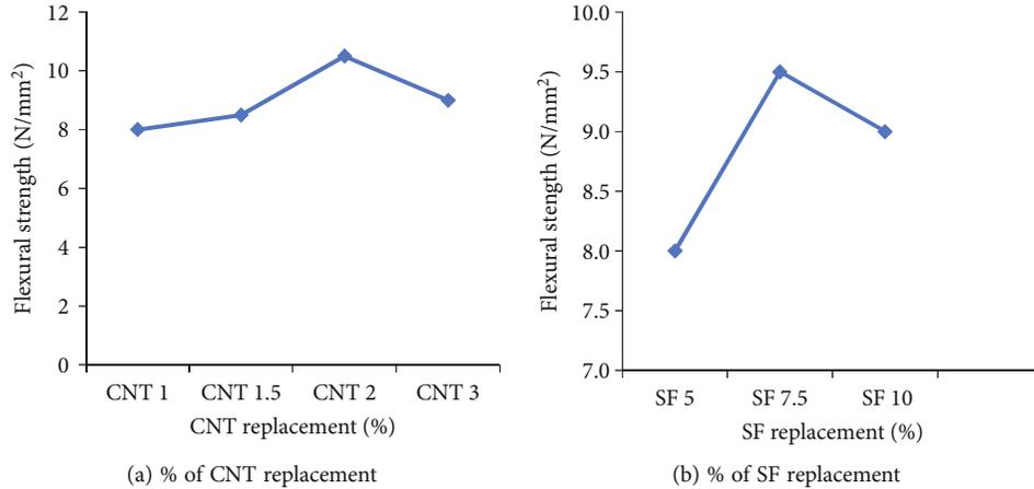
FIGURE 8: Variation of flexural strength at the 28<sup>th</sup> day.
