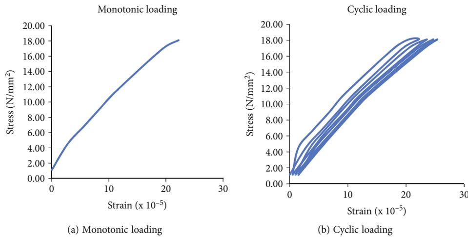
FIGURE 11: Stress-strain curve for 1% of CNT.
