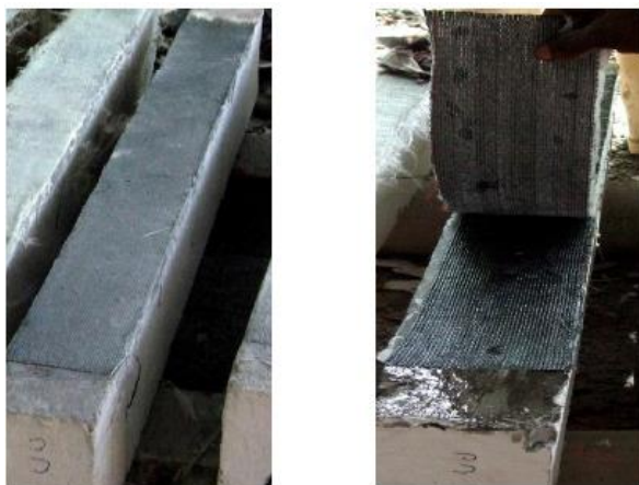
Figure 6. First and second layer of CFRP.
