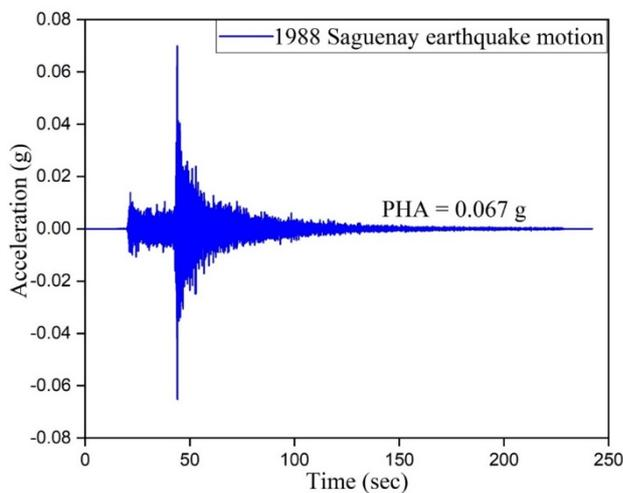
Fig. 11. Illustrates the acceleration vs. time history of input motion.
