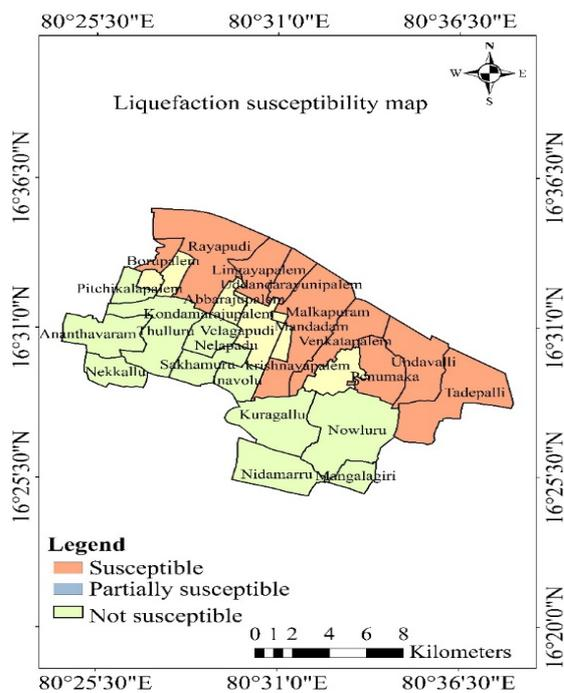
Fig. 17. Liquefaction Susceptibility Map of the Amaravati Region
