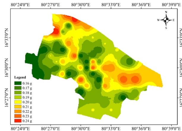
Fig. 16. Spatial distribution of PGA at the surface level
