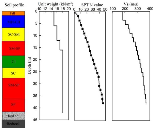
Fig. 6. Soil profile with shear wave velocity, and SPT-N variation
